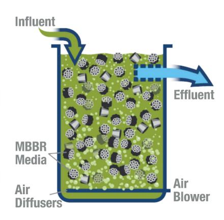
Additionally, the biofilm attached to the mobile bio-carriers within the system automatically responds to load fluctuations.
