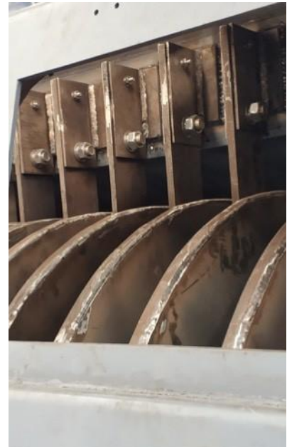
Steel knives to prevent material clogging between discs
