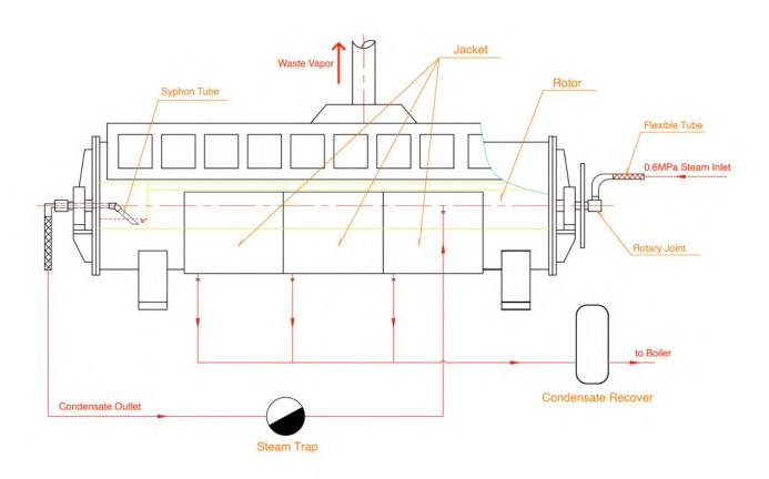
QY series sludge dryer uses saturated steam as heat source (rated steam pressure 0.6MPa), which belongs to indirect steam dryer. It is mainly heated by the main shaft, and can also be heated through the interlayer of the outer casing. The spindle speed is slow, usually 10 to 12 rpm.
