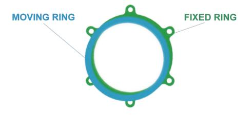
The series of finely machined fixed and moving rings placed alternately provides efficient filtration that remains clog free due to the continuous movement of the rings. This eliminates the needs for consumables like filter cloth etc.
